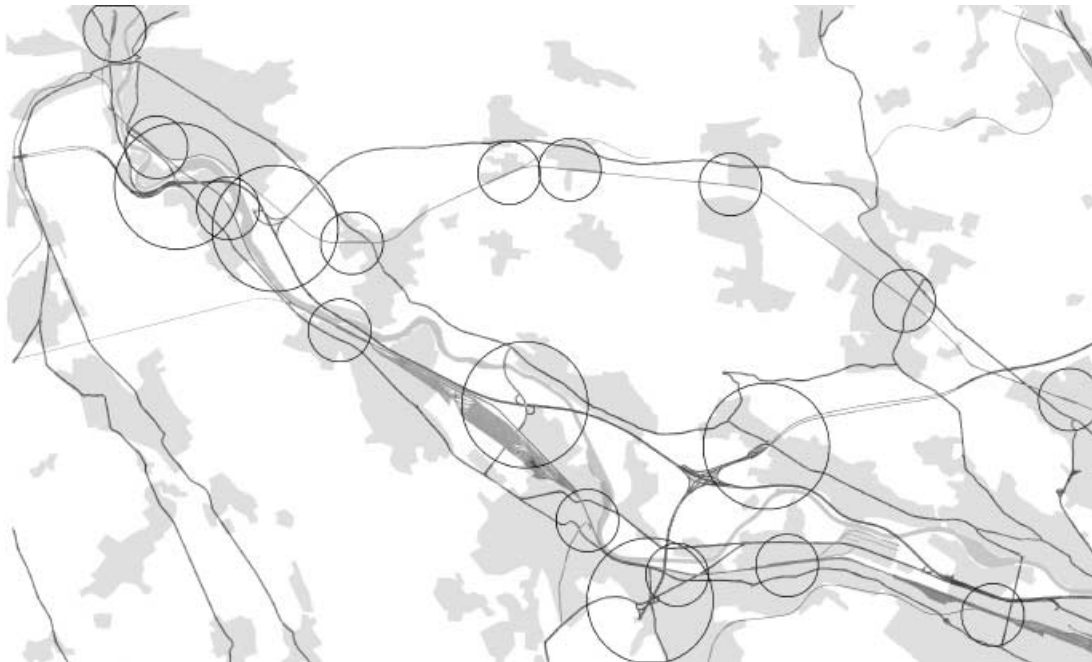
Catchments area of commuter railway stations (radius of 500 m) and motorway entrances/exits (radius of 1000 m)
